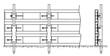
**Step 4:** For vertical curb or partially battered curb, use overhead hangers. (5 per 12' setup)
