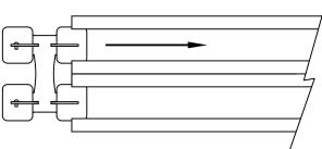
**Step 2:** Set the first two forms in place for the Back of the curb. Drive the stakes through the pockets.
