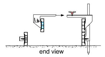
Forming 8" curb face: set face with stacking pockets and stakes.
