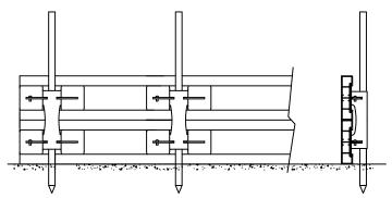
**Step 3:** Set the top form, with slide pockets already in place, through the stakes and into the top position.
