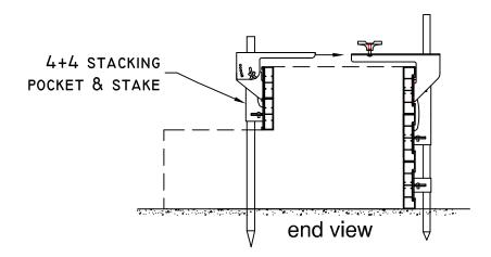
**Step 5:** Complete Setup: Five (5) overhead hangers per 12-foot set-up.
