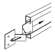
Step 2: Add twist pockets anywhere along the form where additional support is required. *Note: recommend 3 foot spacing.*
