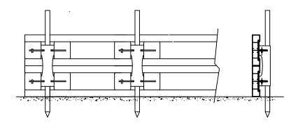
**Step 2:** Set the "front" form at the specified location; install a hanger into the "back" form.
